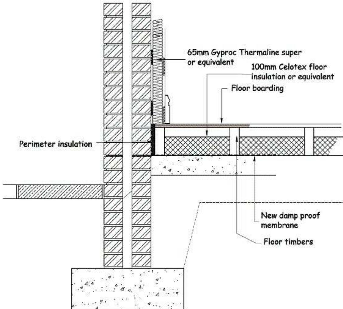
**Cavity Wall with Thermal Laminate**
