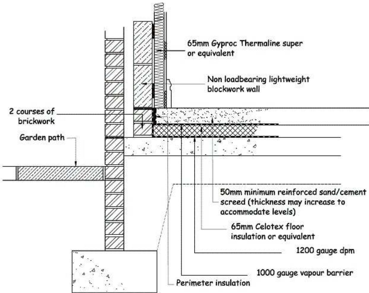
**New Inner Wall & Thermal Laminate**
