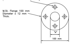
Details of Alternative Wall Mounting Flange to be Used Instead of Column Clamp
