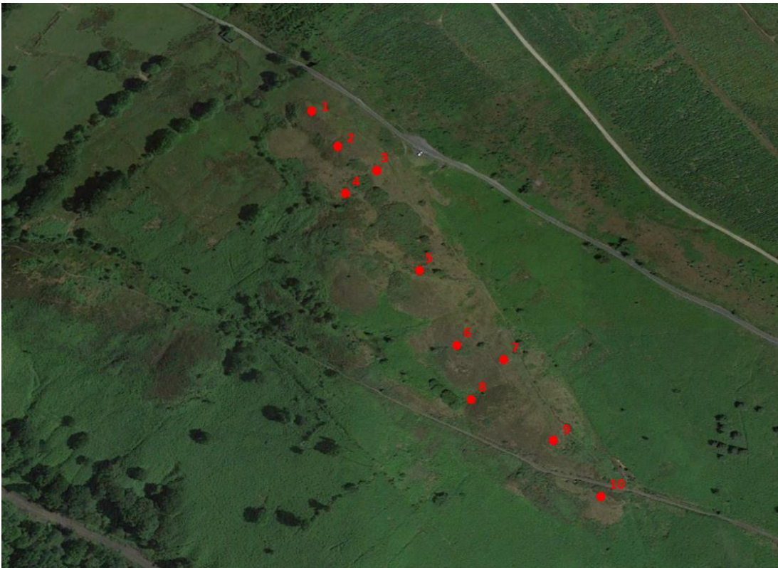
Plan showing fill sampling trial pits taken as a traverse across the slide
