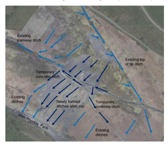
Figure 2.6 – Donor Site (post slip) - Existing surface water drainage features
