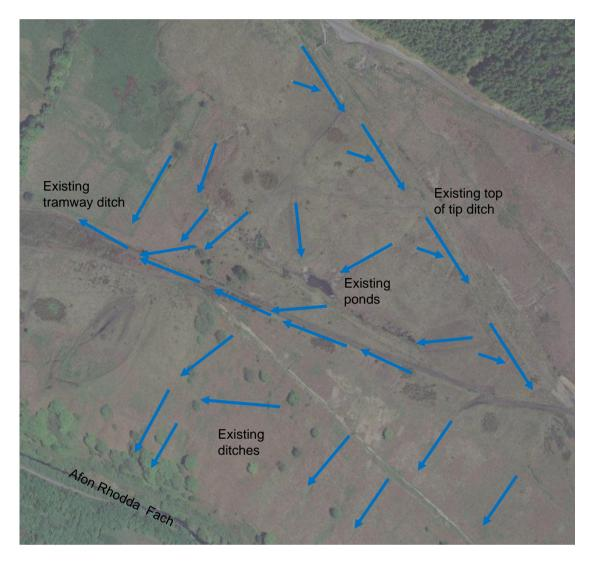
Figure 2.5 – Donor site (pre-slip) - Existing surface water drainage features
