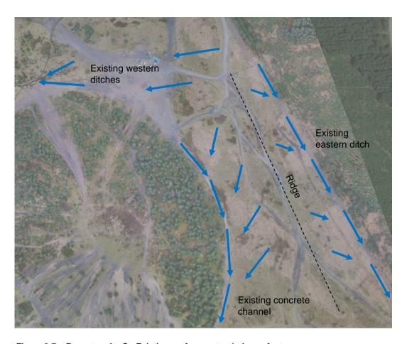
Figure 2.7 – Receptor site C - Existing surface water drainage features
