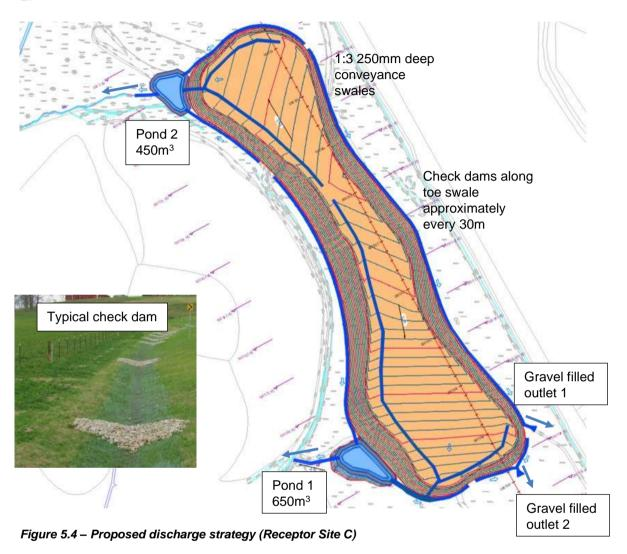
For receptor site C, central swales have been incorporated to convey flows from the top of the deposited material and toe swales to convey flows from the banks. The swales convey flows into two attenuation ponds which discharge into the existing ditches at Greenfield rates via a filter drain connections. Overflow weirs have been incorporated if the filter drains become blocked.
