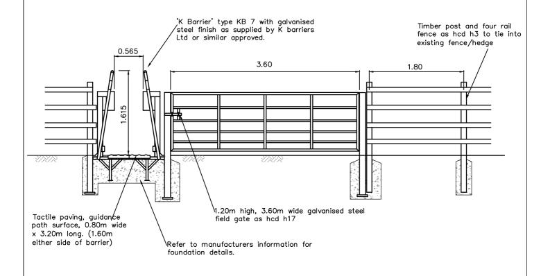
GENERAL ARRANGEMENT OF 'K BARRIER', TYPE H17 GATE AND TYPE H3 FENCE.
