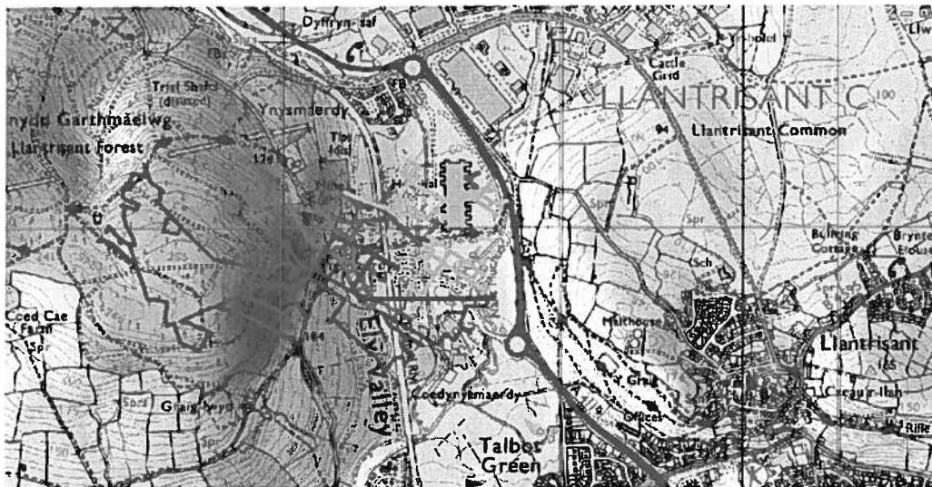
Figure 3: Location of mine workings from Llantrisant Colliery in relation to the surface. The different colours represent separate seams.
