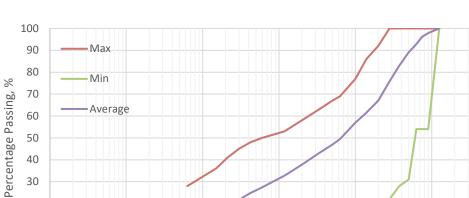
Figure 5.2 – Grading Envelope in Phase 5 Made Ground
