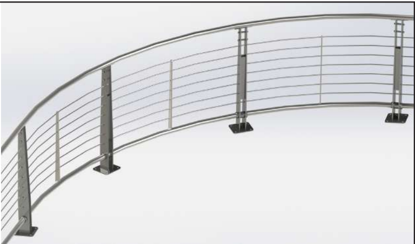
The image is a typical illustrations by the manufacturer showing how they would address the curvature and incline of the handrail system. The specification would be a modified raked upright post, with 10mm Dia or 12mm Dia solid infill curved bar replacing the wire infill. Depending on the span of the upright posts, there would be a central support to prevent distortion.
