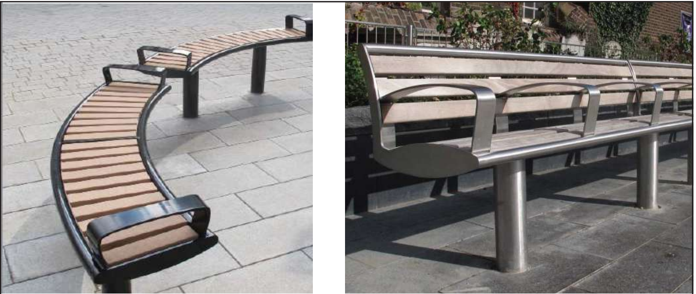
Furnitubes benches Zenith series as specified for the former Bingo Hall site steel frame and posts for in-ground fixing, hot dip galvanised and polyester powder coated, with iroko timber slats smooth planned finish.
