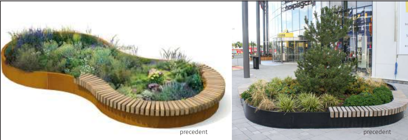
'Streetlife Rough&Ready Free Form Tree Isles' to act as 'central piece' to public realm. Seat: timber, untreated FSC® 100% Hardwood (Louro Gamela) beams (7x15cm | 2.8x5.9") Walls: laser-cut weathering steel class A non-treated 4mm thickOptional: double powder coated finish in RAL colour
