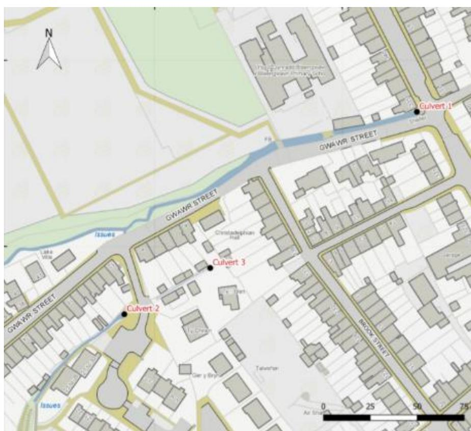
Figure 3: Culvert Inlet Location Plan
