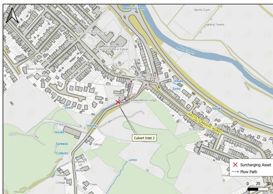
**Figure 7:** Observed flow path as a result of 'Culvert Inlet 2' surcharging during Storm Dennis (15-16<sup>th</sup> February 2020)
