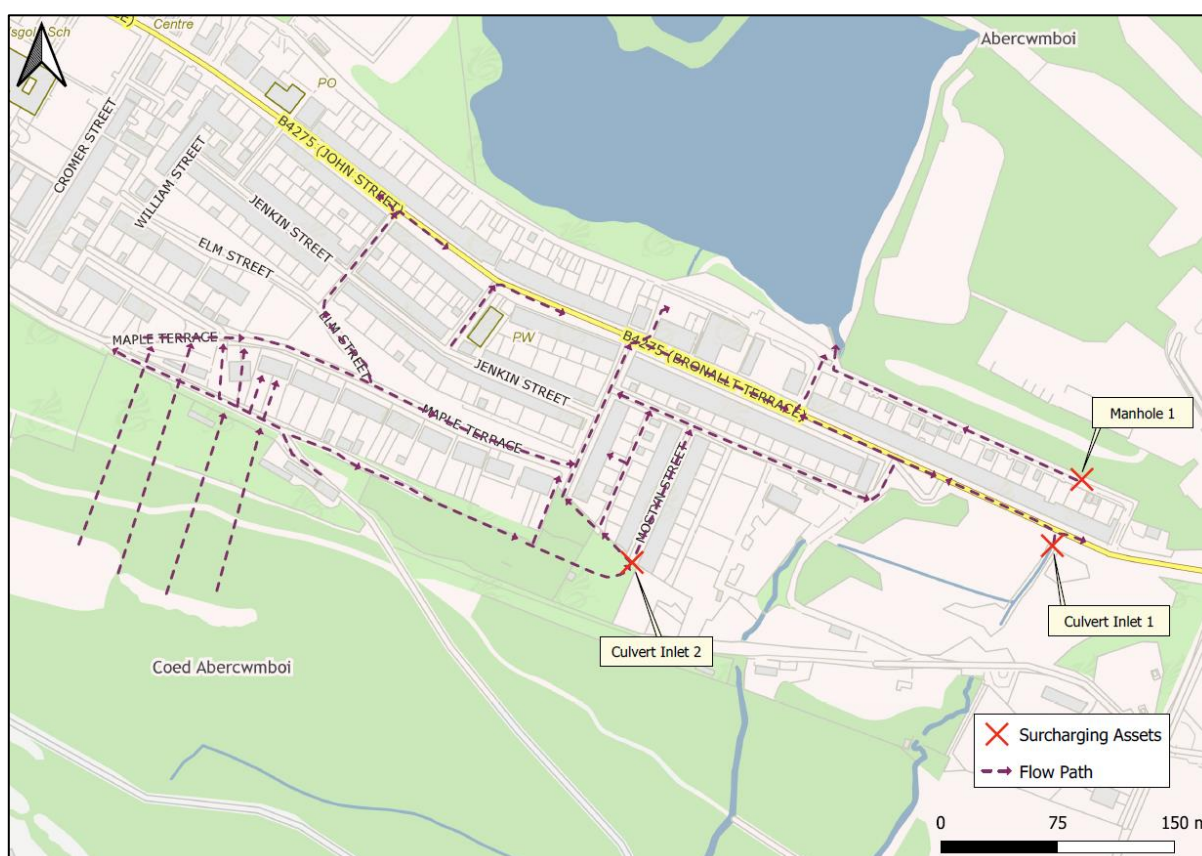
Figure 4: Observed flow paths within 'Abercwmboi' sub-catchment during Storm Dennis (15-16 th February 2020)
