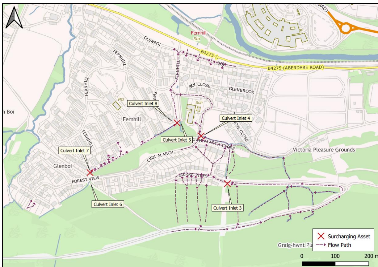
Figure 9: Observed flow paths within 'Fernhill & Glenboi' sub-catchment during Storm Dennis (16 th February 2020)
