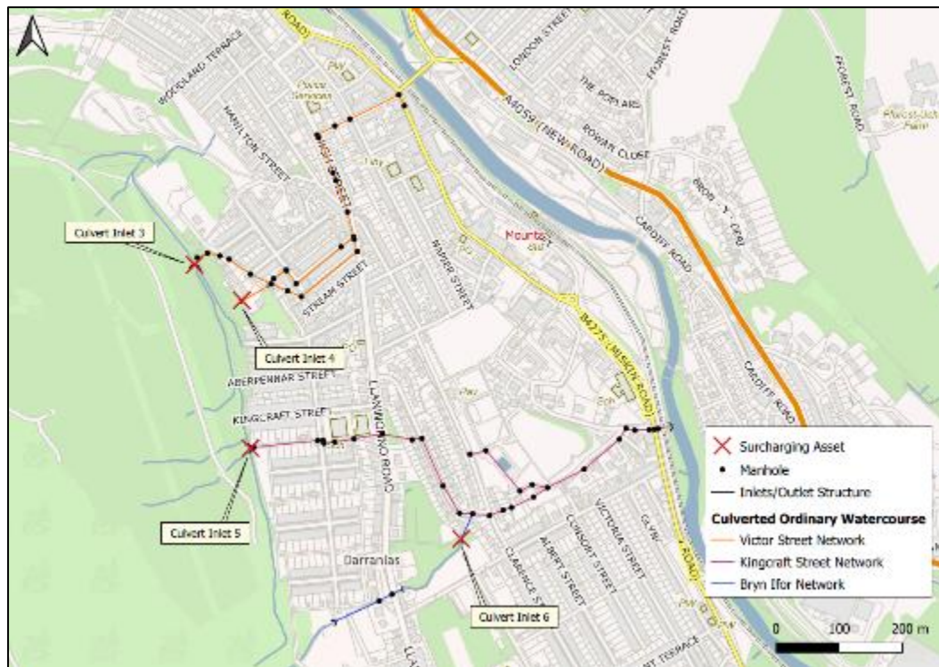
Figure 21: Surveyed culverted ordinary watercourse networks and the infrastructure identified as surcharging within the ‘Mountain Ash West’ catchment.
