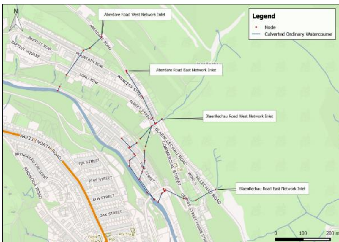
Figure 5: Surveyed culverted ordinary watercourse networks within flood investigation area RCT21
