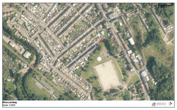
Figure 8: Location plan illustrating the location and flow path of flood water from the manhole within Pleasant Street Park
