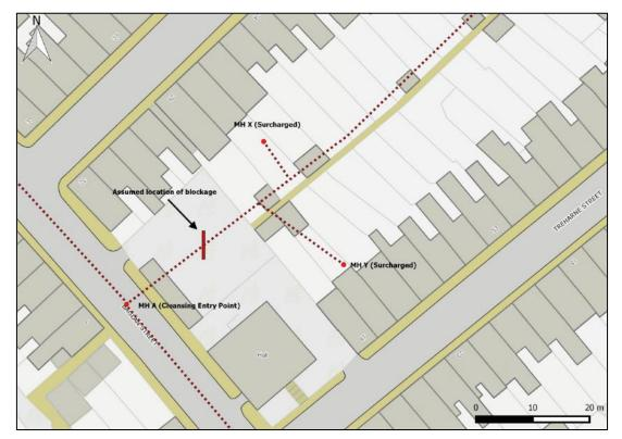
Figure 11: Location of surcharging manholes causing internal flooding to three properties during the 5<sup>th</sup> August 2020 flooding event
