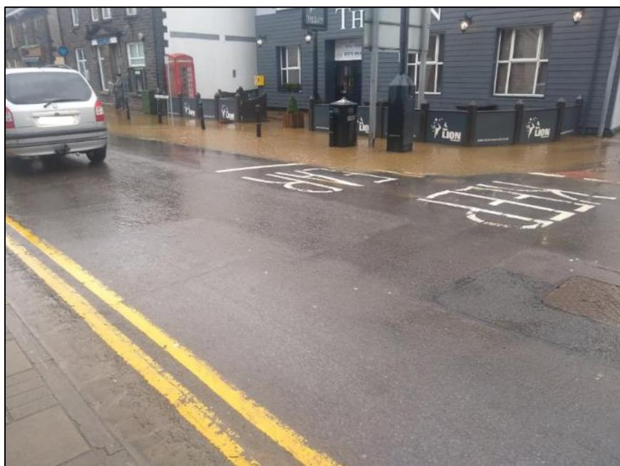
**Figure 6:** Surface water ponding along the A4061 High Street during Storm Dennis on 16<sup>th</sup> February 2020 (image provided by resident)
