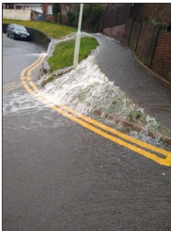
**Figure 8:** Surcharging flows down Heol Tyle Du from 'Culvert Inlet 3' during Storm Dennis (image provided by resident)
