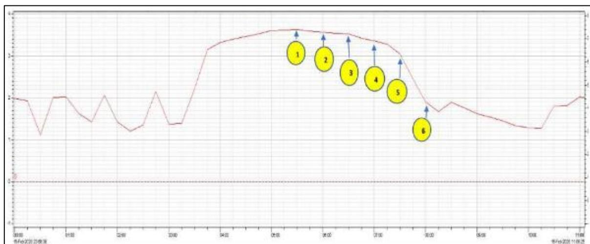
**Figure 19:** Graph showing pumping station levels at 'Trehafod Road Pumping Station' during Storm Dennis (Supplied by DCWW)
