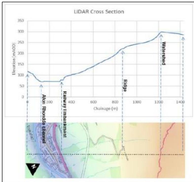
**Figure 3:** Partial Cross Section of the Rhondda Valley, based on LiDAR
