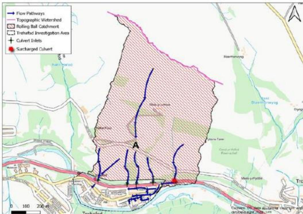
**Figure 4:** Topographic Catchment of RCT18 and corresponding flow pathways (1)
