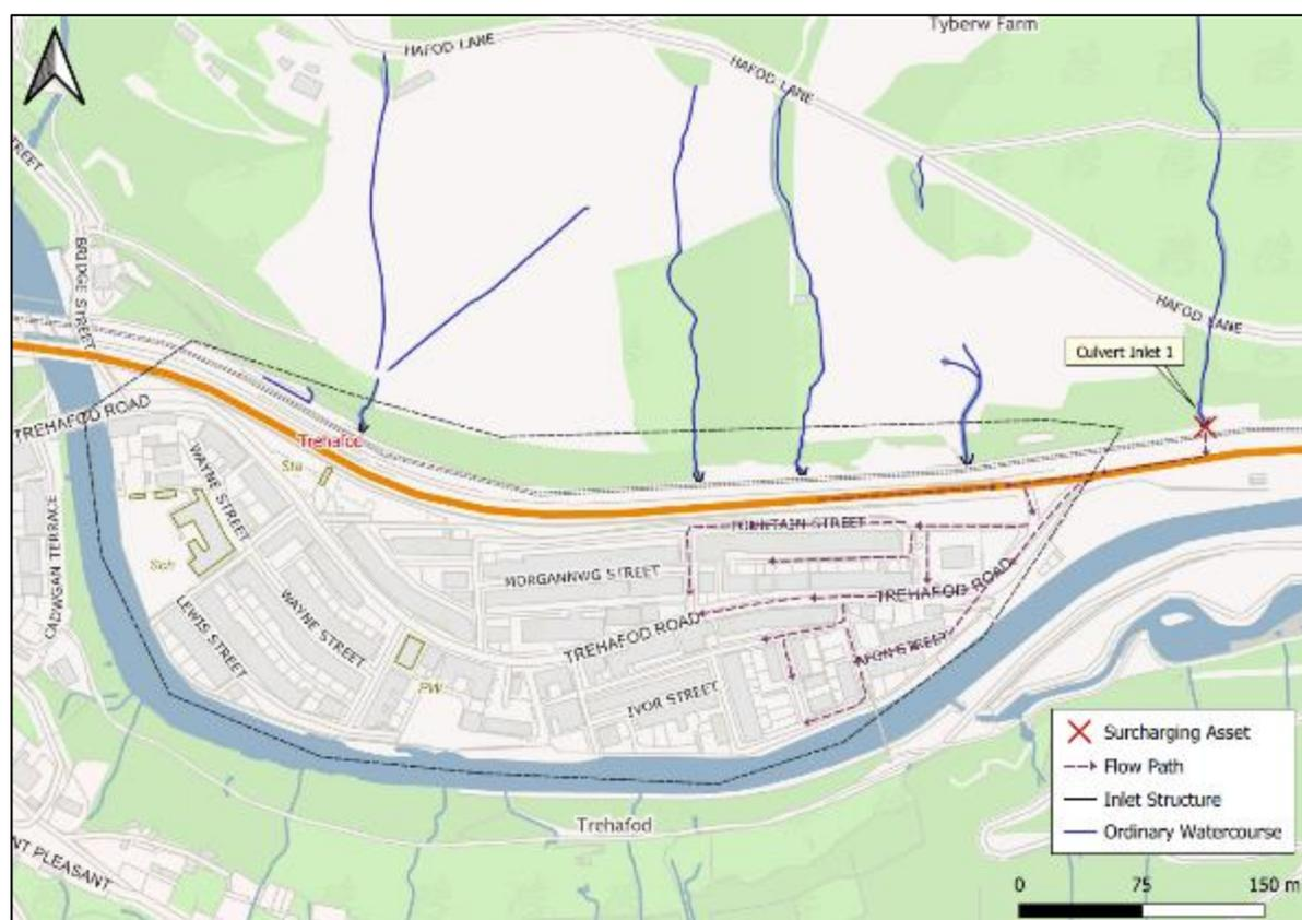
**Figure 5:** Observed flow paths within RCT18 during Storm Dennis (15-16<sup>th</sup> February 2020)
