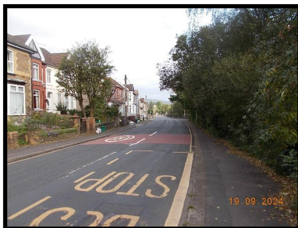
Photograph 4.30 & 4.31 – Overhanging vegetation narrowing the usable footway width along the B4595 Llantwit Road
